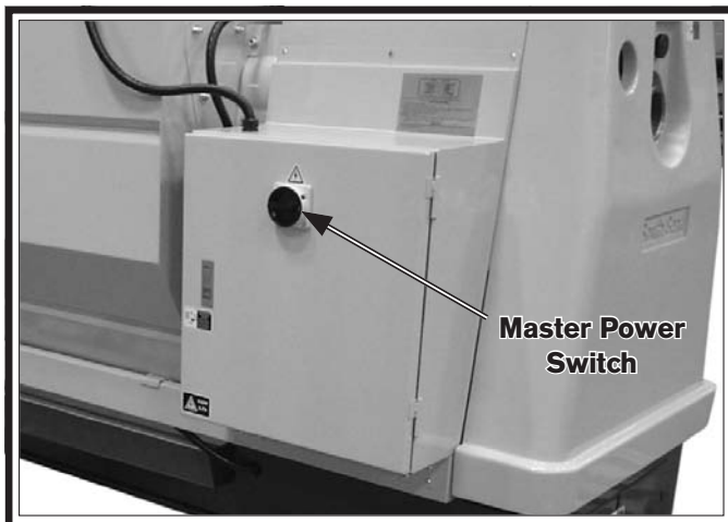
Figure 24. Location of the master power switch.
